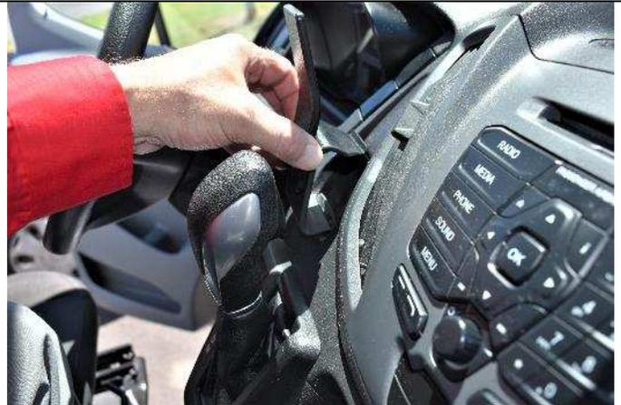
(2) Remove the covering from the tape. Insert the thin lower edge of the mount into the lower seam. Between the dash panel and the rubber compartment insert. See Photo.
