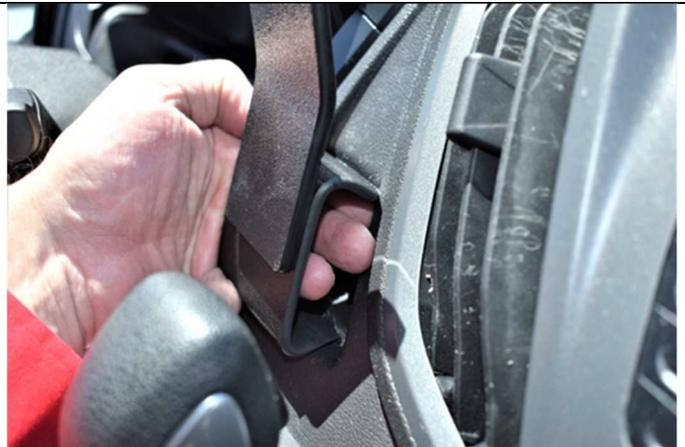
(4) Press up on the top edge to make sure the edge of the mount goes all the way into the seam until the tape touches the dash panel. The tape will not leave any residue if the mount is removed in the future.
