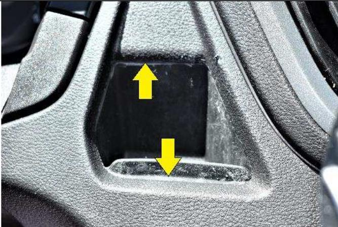
(1) Clean the area where the mount will attach. The mount will attach into the two seams illustrated with the arrows in the above photo.
