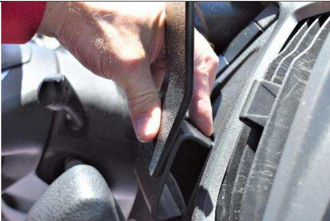
(3) Flex the top of the mount down and insert the thin top edge of the mount into the top seam. Between the dash panel and the rubber compartment insert.
