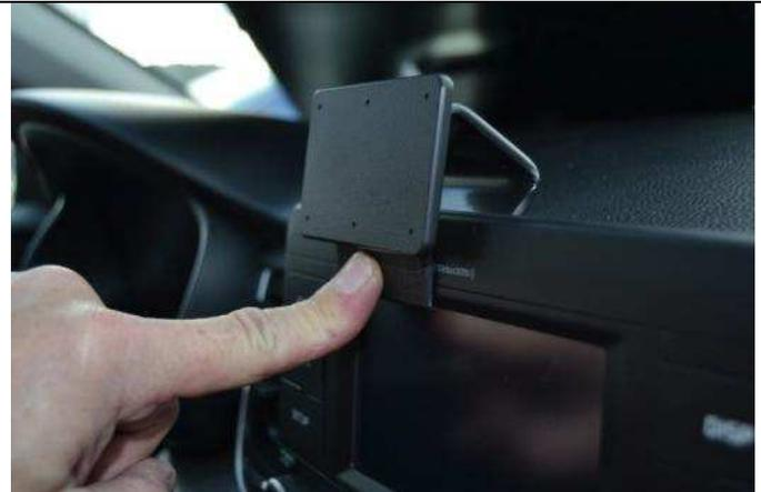
(4) Press in on the mount to make sure the tape connects. The tape will not leave residue when the mount is removed.
