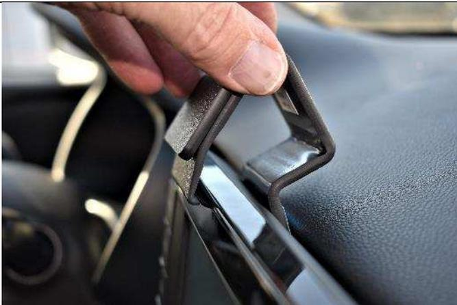
(1) Clean the area where the mount will attach. Remove the covering from the tape. Insert the front "Z" shaped edge into the space between the back of the display and the dash top. The tape on the mount should be facing up/forward.
