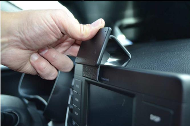
(3) Pull towards you on the face of the mount to flex the lower edge of the mount further down and under the display frame next to the display screen.
