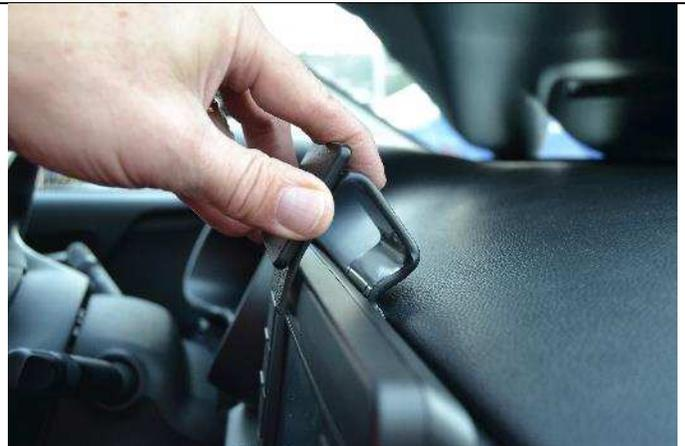
(2) Rotate the mount down so the face of the mount slides over the face of the display frame. The lower edge of the mount might slide into the small seam in the display face.
