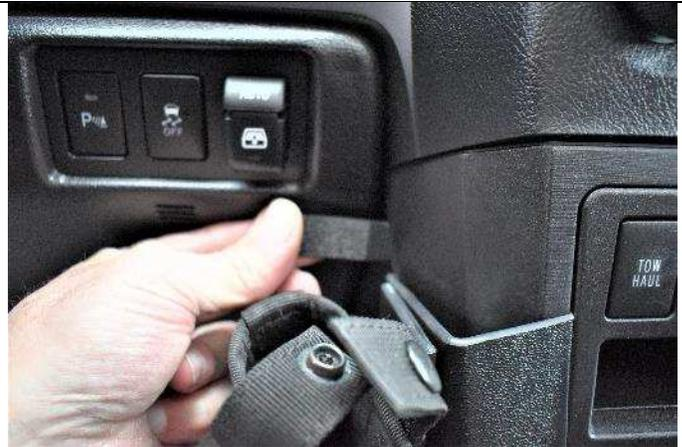
(5) Open the forward seam with the seam tool and press the forward edge of the mount into the seam.
