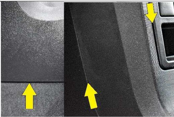
(4) Inspect the area the SAMS will attach to ensure it will not be an obstruction. Clean the area where the mount will attach under the left console side wall. The bottom of the mount will attach under the left console side wall. The two upper edges will attach into the two upper seams illustrated with the arrow in the photo.
