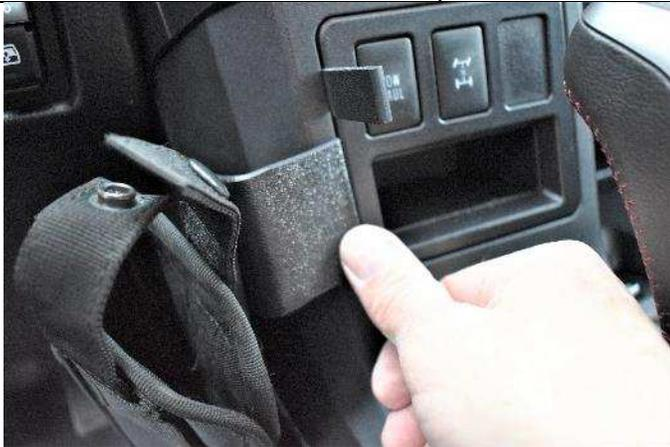
(4) Lift the top of the mount up and press the thin right edge of the mount into the right seam. Use the seam tool to open the seam a little if needed.
