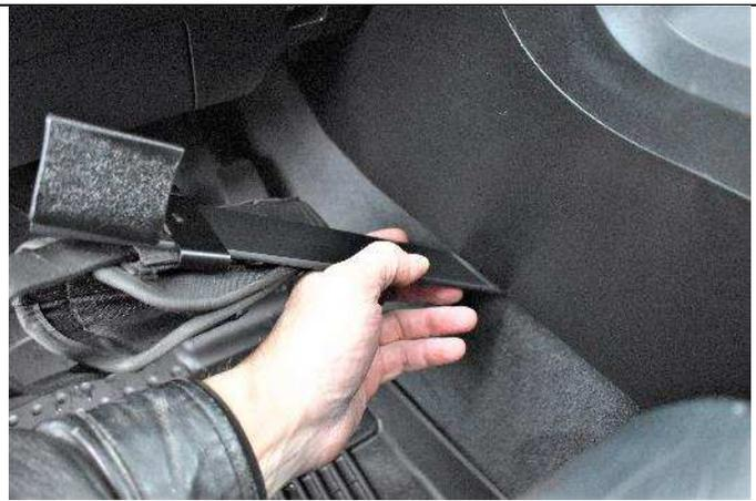
(5) Remove the covering from the tape. Hook the lower "J" shaped edge of the SAMS under the left console side wall. (See Photo)
