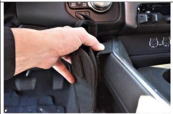
(4) Inspect the area the SAMS will attach to ensure it will not be an obstruction. Clean the area where the mount will attach. Remove the covering from the tape. Press the thin right edge of the SAMS into the seam illustrated in photo 4. (See Photo)
