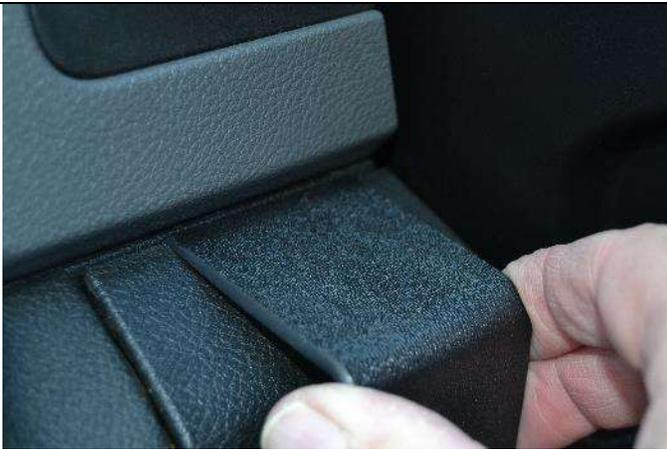
(4) Open the seam just enough to insert the thin upper edge of the mount into the opened seam. (See Photo) The tape will not leave any residue if the mount is removed in the future.
