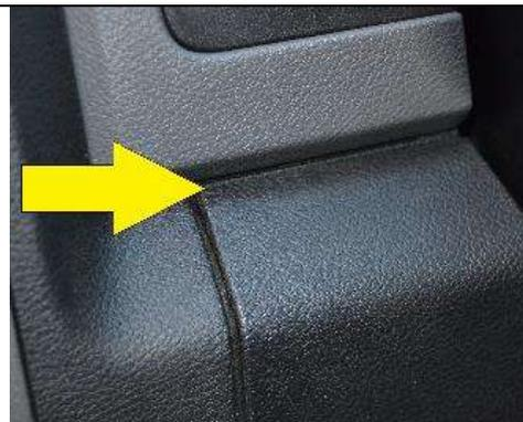
(4) The top of the mount will attach into the seam illustrated in the photo to the left. It is to the left of the steering wheel and between the upper and
