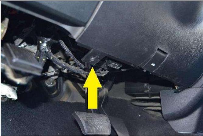
(4) The lower side of the mount will attach with a screw that holds the bottom of the dash panel to the truck frame. See arrow in photo. Remove the screw with a Phillips screw driver.
