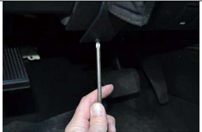
(5) Flex the mount down so the hole in the bottom of the mount aligns with the hole the dash screw was removed from. Securely fasten the mount and dash panel back on with the screw.
