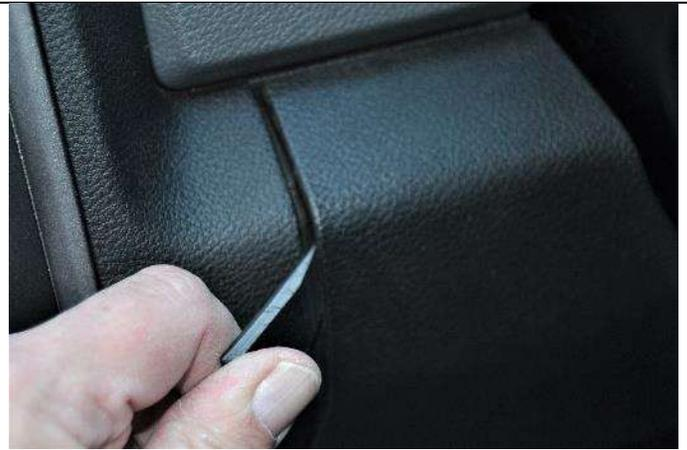
(5) Inspect the area the SAMS will attach to ensure it will not be an obstruction. Clean the area where the mount will attach. Remove the covering from the tape. With the included seam tool gently press the dash panel open.
